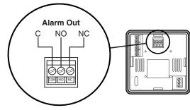
Figure 3.14 Alarm Connections
